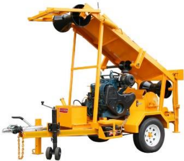
Sewer cleaning bucket machine
