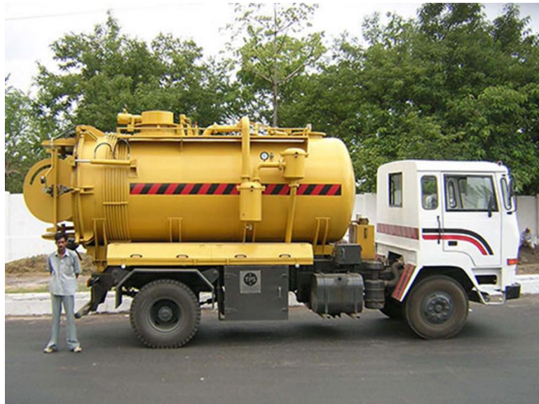
Hydro Jetting Machine
